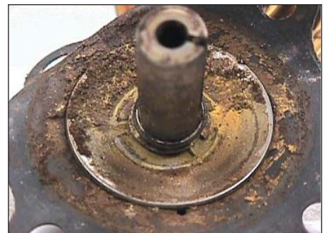
Any contaminants that are not filtered from the compressor will eventually wind up in the machinery or end product
